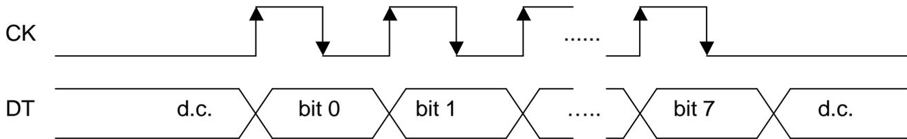
The clock and data lines include a series resistor of 470 ohms at the decoder and on the SUSI-module. The data line must have a pullup resistor to 5 V of = 15kOhm directly on the decoder's sending device ("before" the 470R). Signal level is 5Volts.
